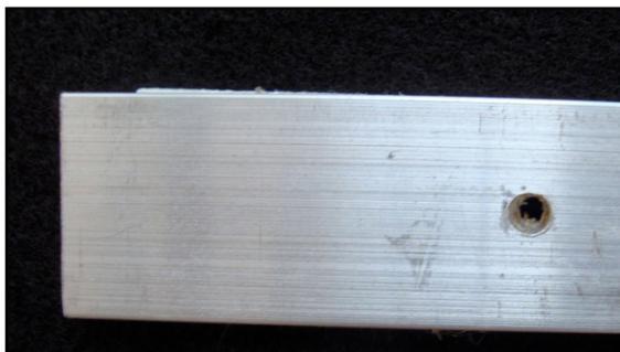
7. Drill the hanging holes in the bar before you attach the bar permanently to the back of the piece. Use an electric drill with a titanium drill bit. The hole can be any size. I usually use 1/8" drill bit. Put the bar on a piece of scrap wood to stabilize it. Drill the hole through the bar and into the wood. The hole should be about 1/2" from the end of the bar.
