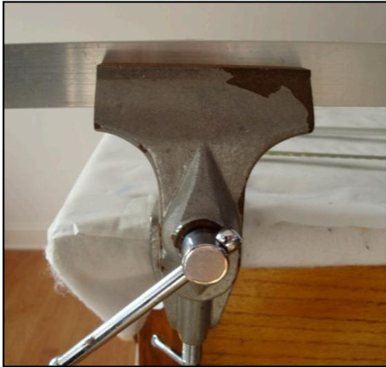
3. Mark the place where the bar will be cut with pencil. Put the bar in the table clamp and use the tightening screw to make sure the bar is stable.
